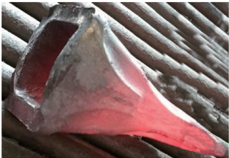
图 18 工艺实验得到的终锻件 Fig. 18 Final forgings obtained from process test
