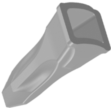
图 9 斗齿锻件三维模型 Fig. 9 Three-dimensional model of bucket tooth forgings
