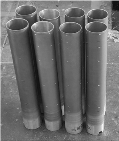
图 6 淬火后旋压成形的内径为 \Phi 60 mm 的薄壁管 Fig. 6 Thin wall tubes with inner diameter of \Phi 60 mm formed by spinning after quenching
