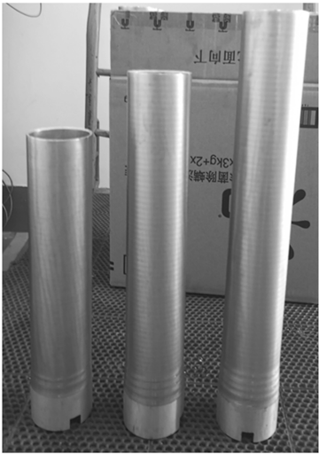
图 5 退火后旋压成形的内径为 \Phi 60 mm 的薄壁管 Fig. 5 Thin wall tubes with inner diameter of \Phi 60 mm formed by spinning after annealing
