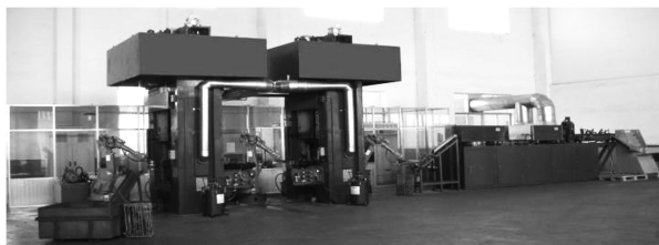
图 2 环保型电动螺旋压力机和精锻自动化生产线 Fig. 2 Environment friendly electric screw press and precision forging automatic production line
