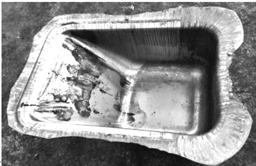
图 12 灰斗拉深优化后成形零件图 Fig. 12 Diagram of forming parts for gray hopper deep drawing after optimization
